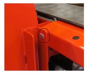
6. Dismount the four marked screws attaching the drive roller bracket. Dismount the bracket allowing access to drive motor and and bearing.
