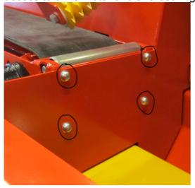
7. Dismount motor and bearing allowing the drive roller to be removed. Remember to loosen the set screw for the bearing as indicated.
