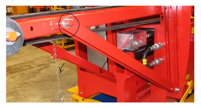
5. Dismount the two screws indicated and remove them. Loosen the feeding belt so that the only obstacle for complete removal now is the drive roller.
